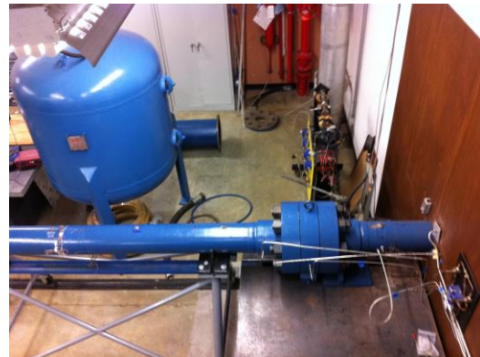
(b) Detonation tube, diaphragm section and Driver tube
